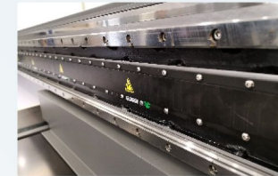
Optional linear motor assures extremely accurate, quiet and stable movement
